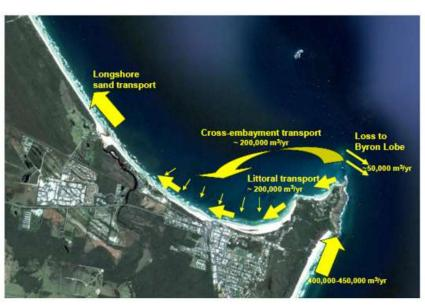
Figure 3.3 Conceptual sand transport (BMT WBM, 2013)
